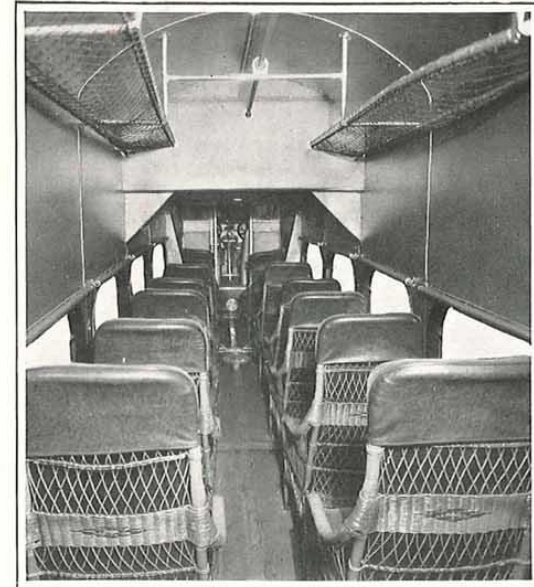
Interior of 14-passenger Ford air liner, standard equipment of Northwest Airways Service.
