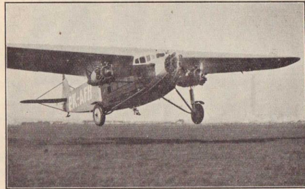
The triple engine Fokker F XII, with room for 14 passengers
