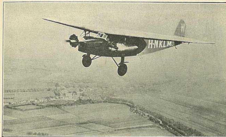
THE FAMOUS FOKKER COMMERCIAL MONOPLANE type F VIII - 2 engines - 15 passengers - speed 110 miles P. H.
